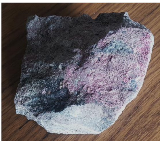
Image 1 (above): Cobalt bloom at Bay Lake, noted by the pink colouration on the rock sample.
